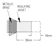
2 Apply RTV-2 sealant generously to the outside of the ET-8 end cap & onto the end of the cable.
