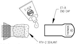
3 Slide the end cap onto the cable with a twisting motion, making sure to work out any air pockets. Wipe off the excess sealant. Pull the braid over the end cap & then crimp together the braid ends with the 8-AWG compression lug supplied.
